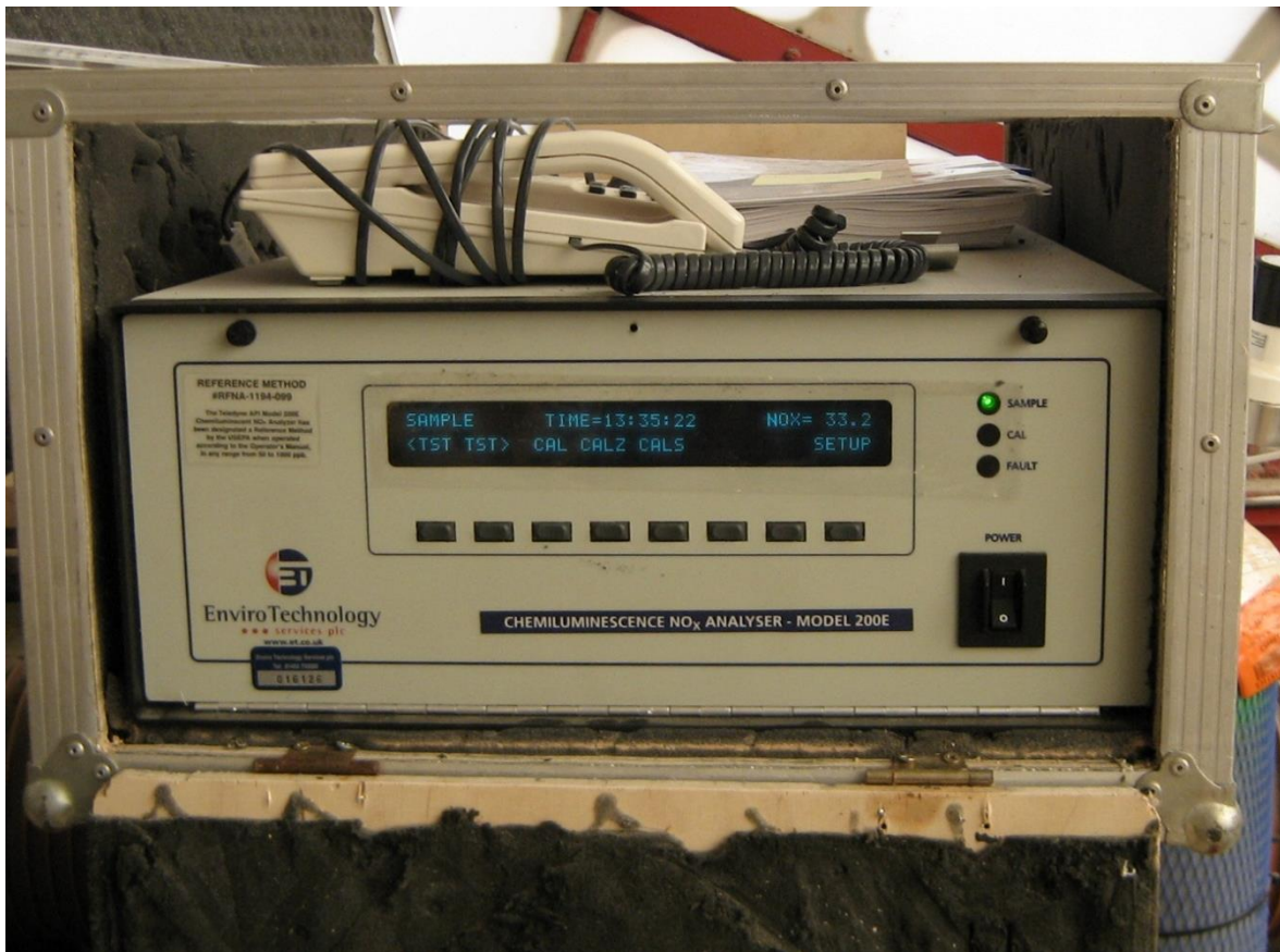
Figure 2-2: Automatic NO x analyser at Halkett Place, St Helier
